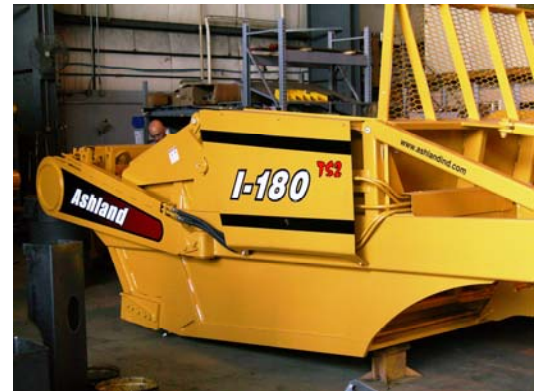
Ashland I-180 earthmover in production
