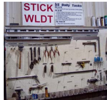
5S shadow board in Genesis Equipment's welding area.
